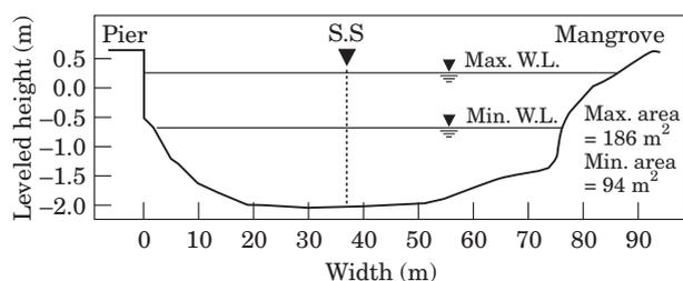
FIGURE 2. The sampling cross section, looking downstream. S.S.: sampling station. W.L.: water level.
